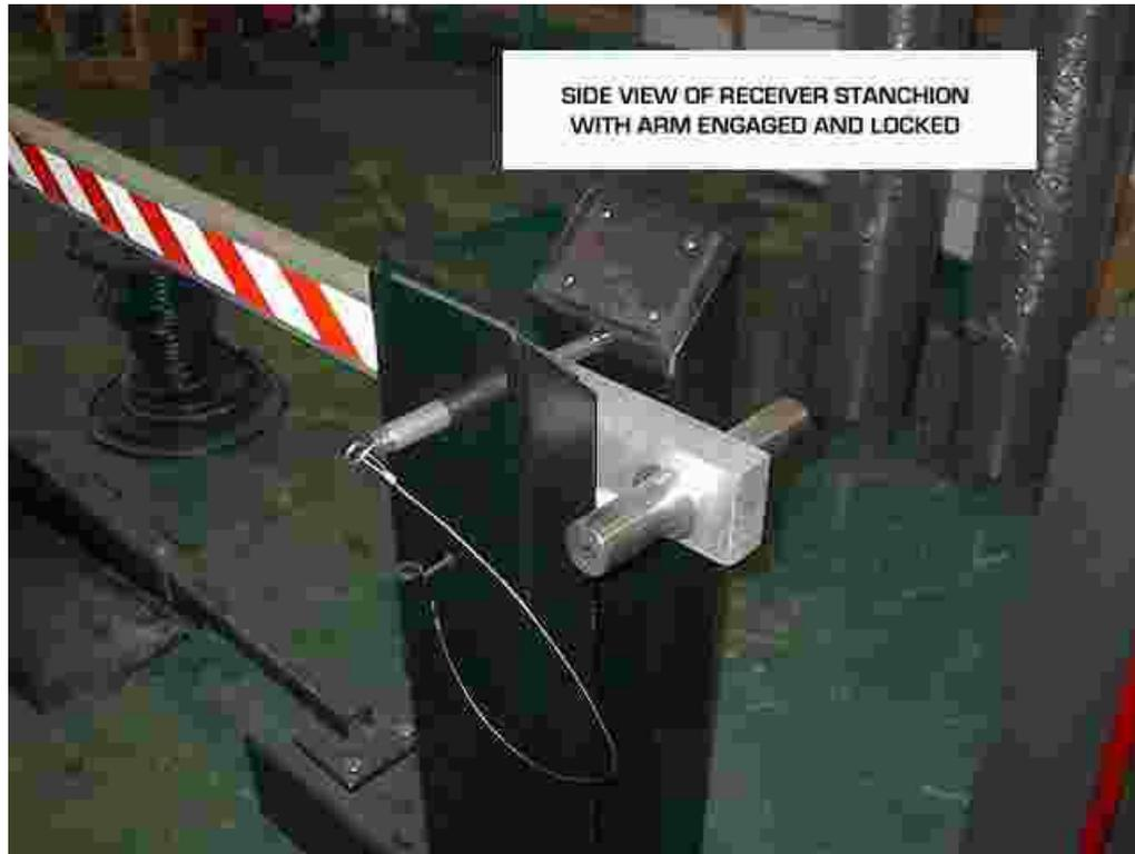
Both the hinge post and receiver post are cast in place in a subterranean concrete pour. Both posts have elevation grade locators to aid the installation. The installation requires no above-grade concrete. The portions of the hinge and receiver posts that are imbedded are coated to prevent deterioration due to cement contact. The aboveground portions of the posts are primed and finish painted in black.
